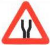
Road Widening Ahead
